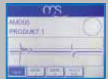
Continuous on-screen signal profile (here with metal detection)
